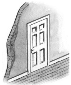
5. A non-load bearing timber stud partition separates two bedrooms on the first floor of a two storey dwelling house, as shown in the accompanying sketch. The first floor joists are 225 mm × 50 mm, the floor is a tongued and grooved floor and there is a plasterboard ceiling beneath. A flush panel door is fitted in the partition.
